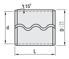
Parts are centered with dowel pins in dies & moulds. After inserting / removing processes, these dowel pins creates gaps and they can be easily inserted / removed. This situation may cause the pin be removed and fall into the die / mould and damage to die / mould parts. In order to avoid such situations, after inserting dowel pin in mounting place, the dowel pin retaining sleeve is attached. It provides safety against falling of pin. It is used as ring in the hole for dowel pins.
